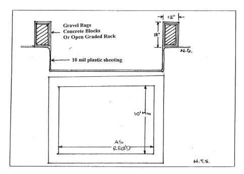
Alternative Self-installed Construction Site Concrete Truck Washout
