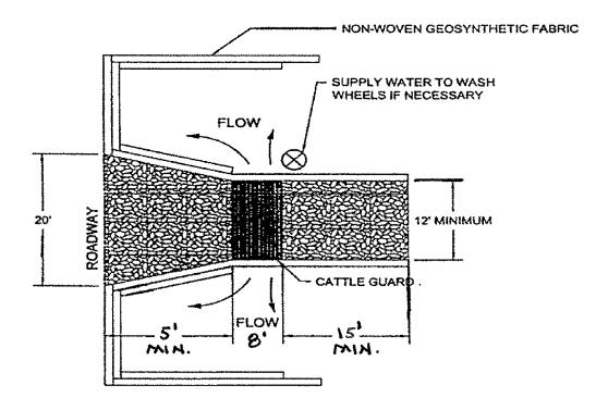
A steel grid that allows the safe passage of vehicles while agitating the tires to loosen and remove the soil build up. The grid or structures shall conform to the following:
